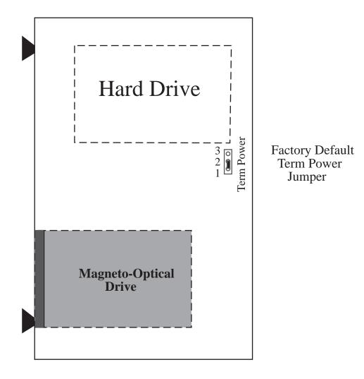
Figure 1-2: VX2-350-SC-DSMO Jumper Configuration
