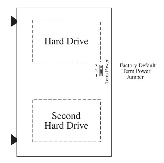
Figure 1-2: VX2-350-SC-DS Jumper Configuration
