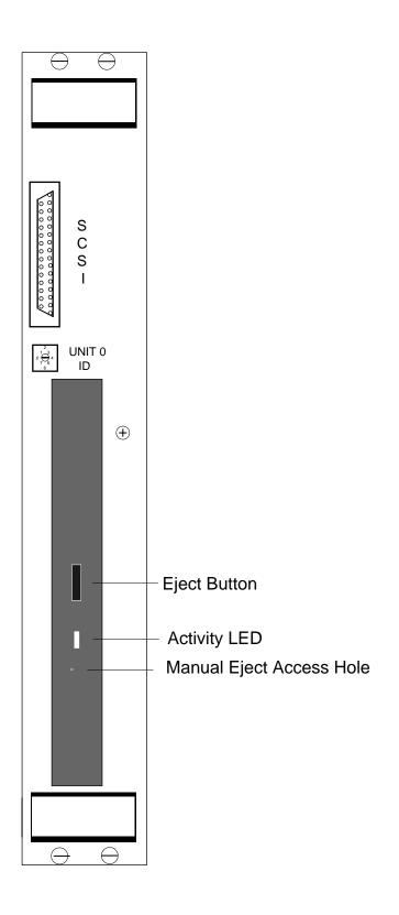
Figure 1-1: VX2-350-SC-CD Front Panel
