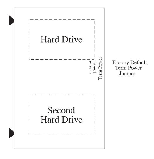
Figure 1-2: VX1-250-SC-D Jumper Configuration
