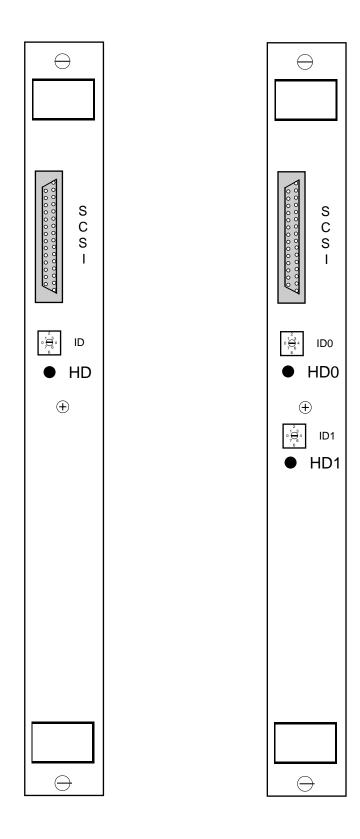
Figure 1-1: VX1-250-SC-D Front Panel
