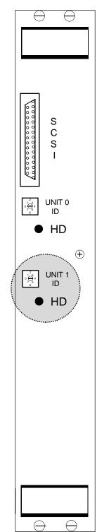
ID Switch and Hard Disk Activity indicator for Second disk drive
